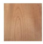
Bio-composite sheet of recycled craft paper is executed with the use of bio-resins made of plant waste from sugar production. Such sheet checked for hazardous substances and with a biological base, is a sample of sustainability. Due to the use of processed and natural materials the client gets a choice between different surface structures of natural brown hues.
