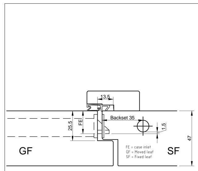
Rebate retracting bolt, locks automatically in upper and lower positions
